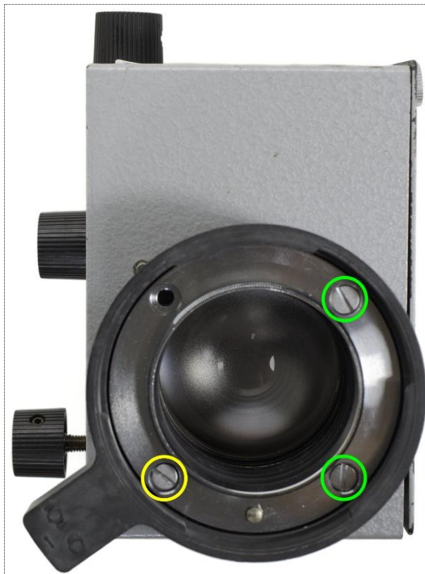
Figure 33: The left-handed configuration of the light port of lamphouse 100.
