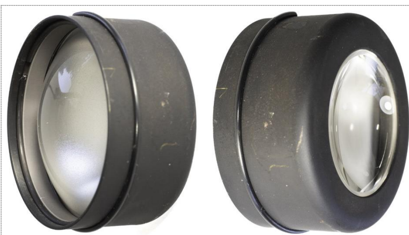
Figure 9: Views from different angles of a collector case after removal from lamphouse 100. The left image shows the side (with a frosted lens) that faces the microscope; the right image shows the side that faces the lamp bulb.
