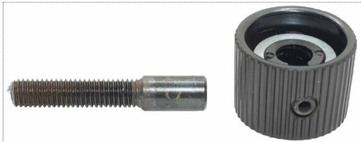
Figure 50: The removed and disassembled horizontal lamp adjustment control.
