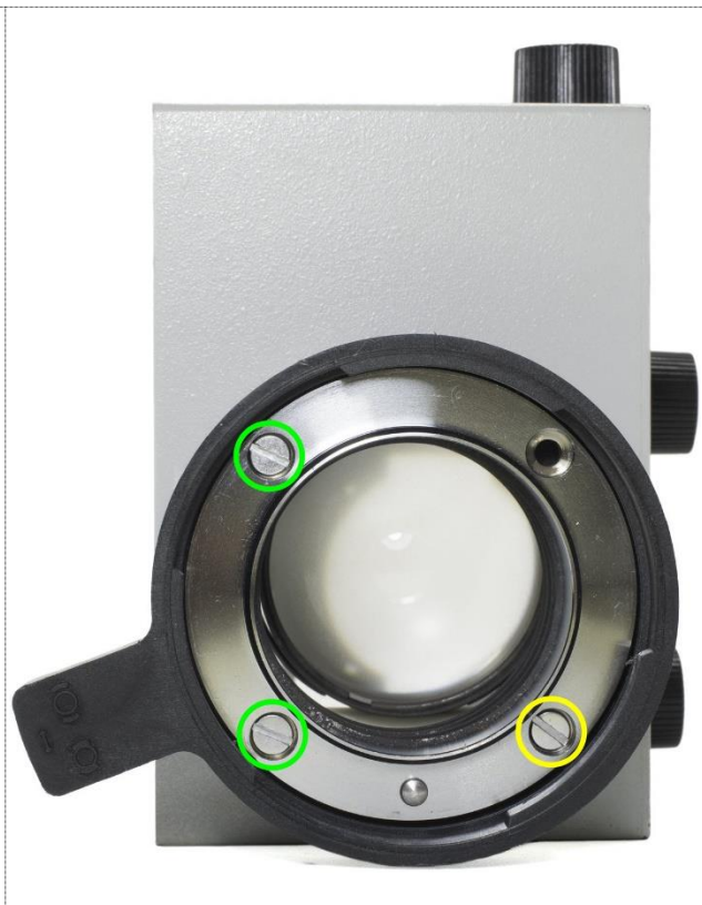
Figure 34: The right-handed configuration of the light port of lamphouse 100.
