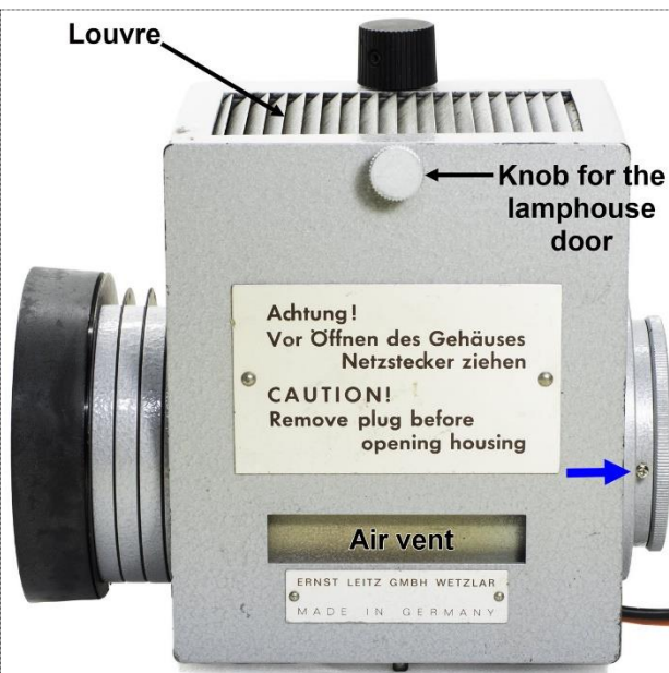
Figure 3: Lamphouse 100 – view of the side with the removable lamphouse door.
