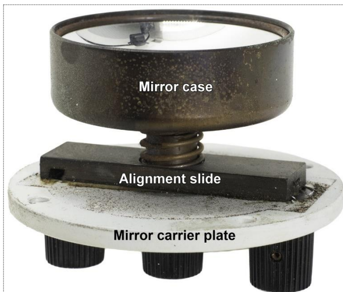
Figure 13: The alignable and focusable mirror after removal from lamphouse 100Z.
