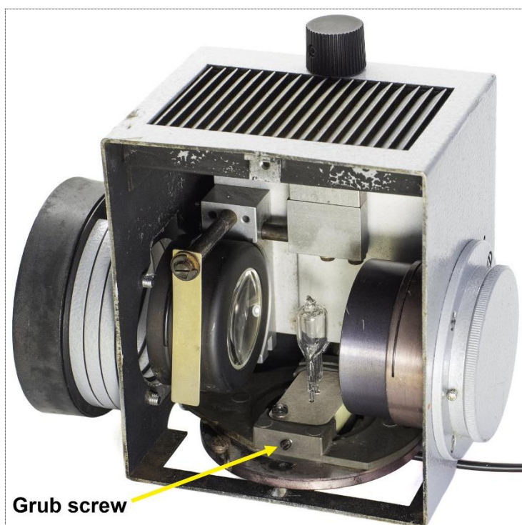
Figure 27: The inside of lamphouse 100 with the halogen bulb holder in the baseplate.
