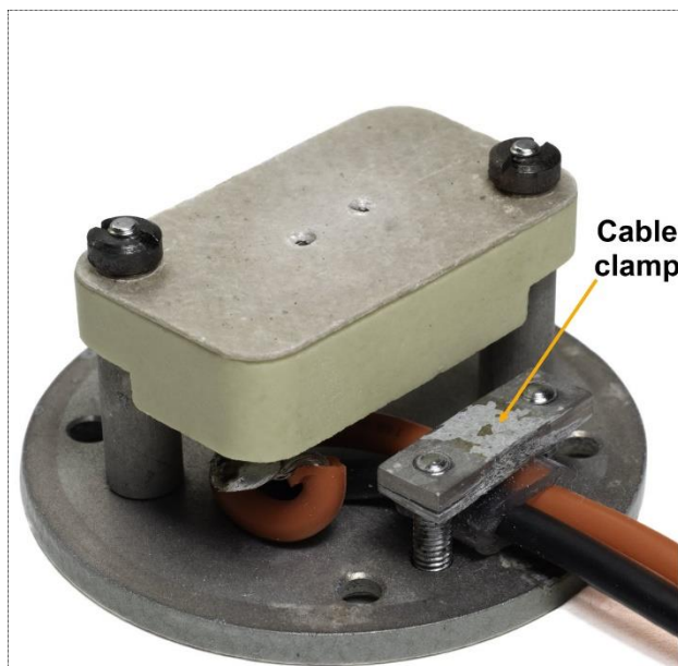
Figure 31: The halogen bulb holder after the case has been removed.
