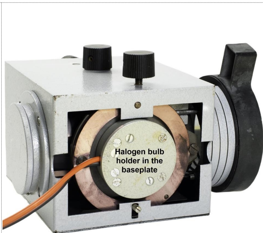
Figure 5: Lamphouse 100 – view of the underside.
